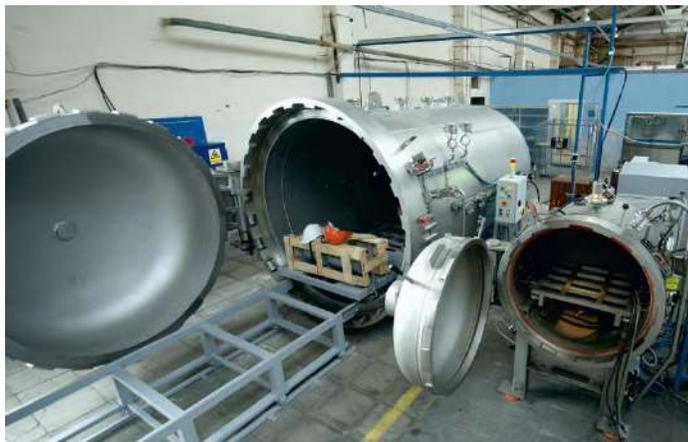
**Device for determining the heat-insulating properties** of shoes when exposed to various negative temperatures (DVT SKY). The shoe sample is placed in a thermal container for a certain period of time, then the temperature of the insole is measured.
