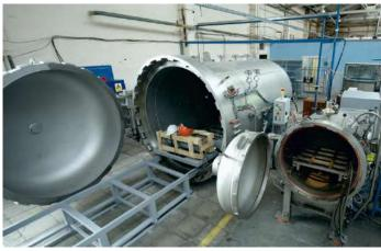
**Device for determining the heat-insulating properties** of shoes when exposed to various negative temperatures (DVT SKY). The shoe sample is placed in a thermal container for a certain period of time, then the temperature of the insole is measured.
